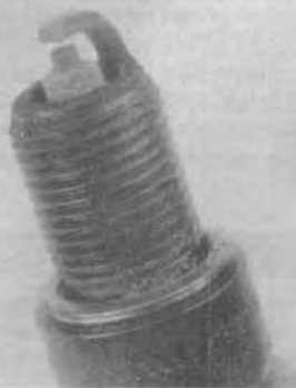
Fig. 6 This plug can be cleaned and re-used
