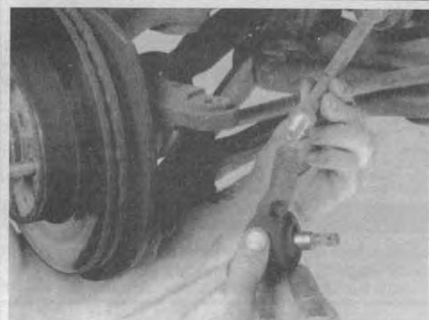
Fig. 59 Here the tie rod end has been removed—a simple matter of unscrewing by hand because the locking nut was previously loosened
