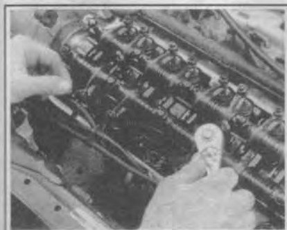
Fig. 56 To remove the rocker arm and shaft assembly loosen, but do not remove the camshaft holder bolts
