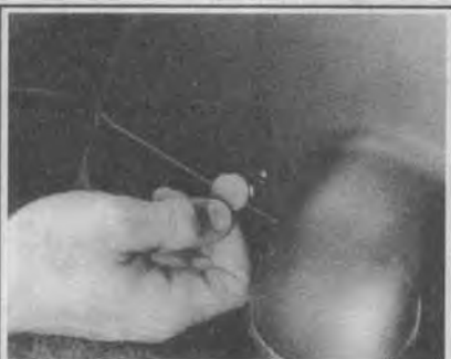
Fig. 37 Remove the trim cap covering the Phillips screw and remove the screw—1984-87 style CRX shown
