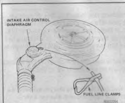
Fig. 83 Clamp off the air intake control vacuum hose—1985-87 carbureted models
