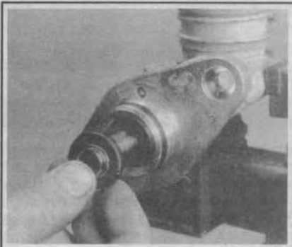
Fig. 12 Remove the outer secondary cup from the master cylinder
