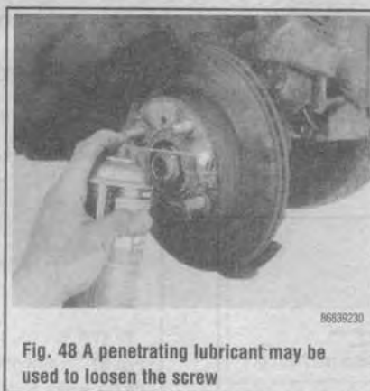
Fig. 46 The (front) rotor as it appears upon removal of the wheel
