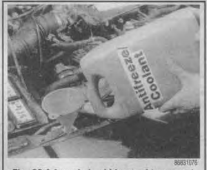
Fig. 96 A funnel should be used to prevent spilling coolant over the engine and painted surfaces
