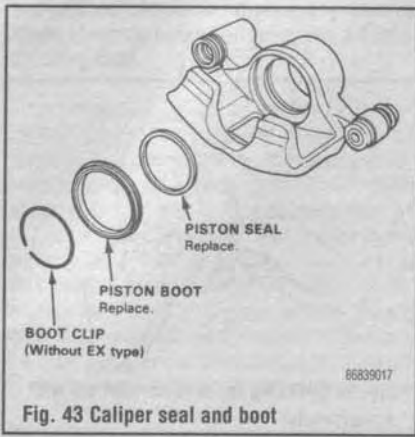
Fig. 44 Proper location of caliper seal, boot and clip
