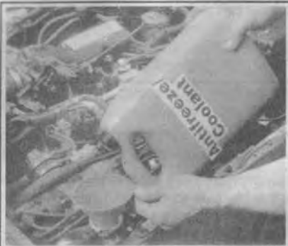
Fig. 94 After the cooling system is drained, fill the system through the radiator
