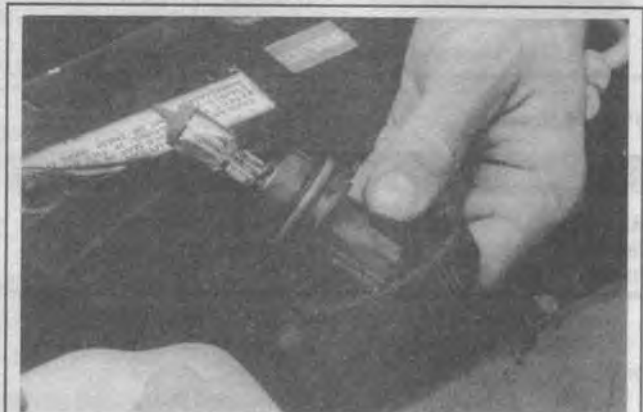
Fig. 72 Removing the halogen headlight bulb from the back of the headlight housing
