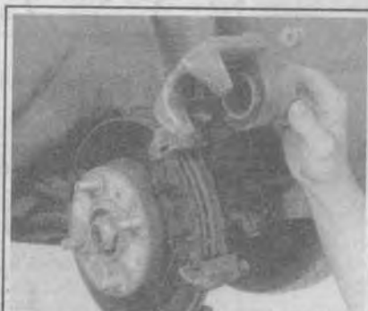
Fig. 28 Pivot the caliper out of the way . . .
