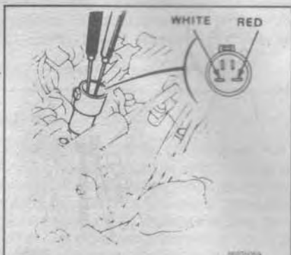
Fig. 41 Crank angle sensor testing—1985-87 fuel injected models
