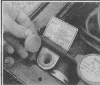
Fig. 95 The cooling system should be topped off through the expansion tank
