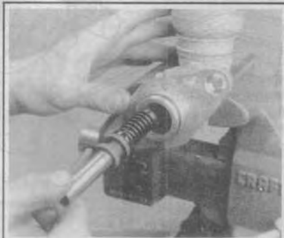
Fig. 16 Remove secondary piston A and B assembly
