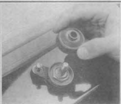
Fig. 53 Check the dust/moisture cap for damage
