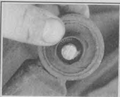
Fig. 43 The lower through-bolt that secured the original shock absorber to the suspension on this 8-year old car was rusted solid and had to be cut off
