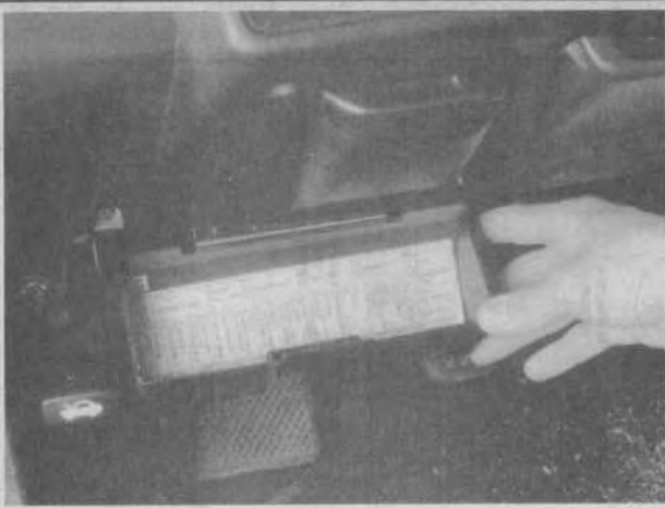
Fig. 86 The fuse box in the car protects many components and includes a fuse puller tool and spare fuse from the factory
