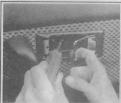
Fig. 44 Removing the door handle trim plate—1984-87 models
