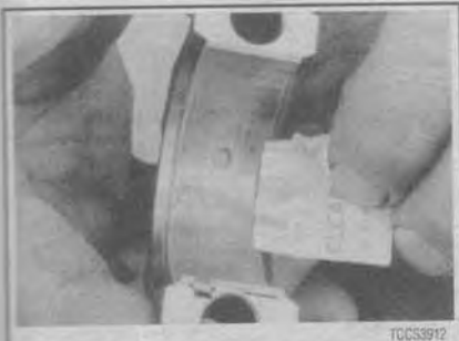
Fig. 173 After the bearing cap has been removed, use the gauge supplied with the gauge material to check bearing clearances
