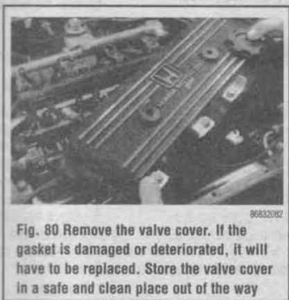
Fig. 77 The first step to valve adjustment is access via the valve cover
