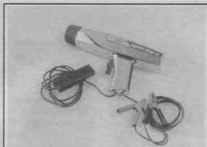
Fig. 11 Inductive type timing light
