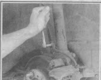
Fig. 10 With the vehicle supported, begin shock absorber removal by detaching the brake hose clamp
