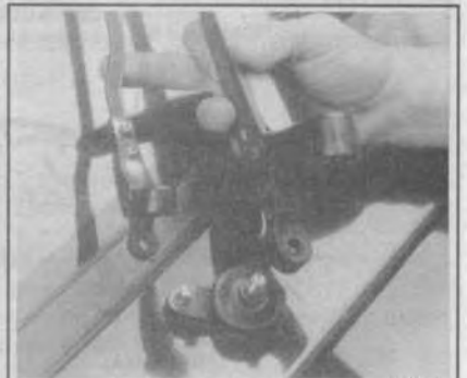
Fig. 52 The rear wiper arm assembly is now free to remove to a safe place
